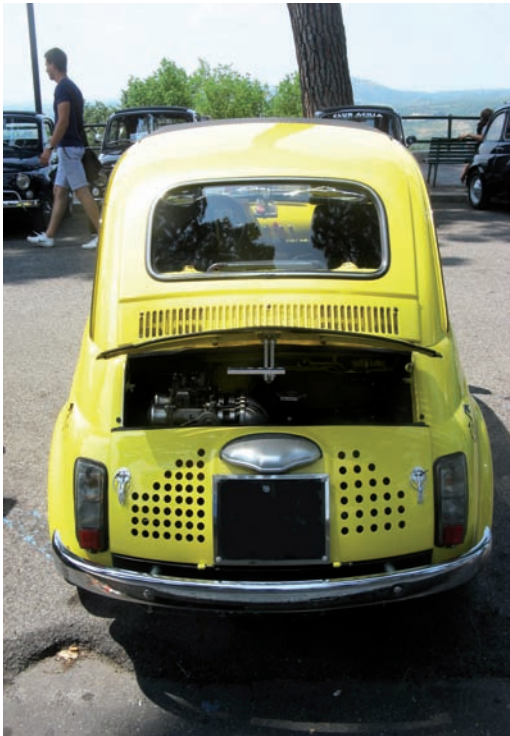
Yellow Fiat 500 Tivoli. Door to engine compartment modified to improve air flow and looks. July 2013
