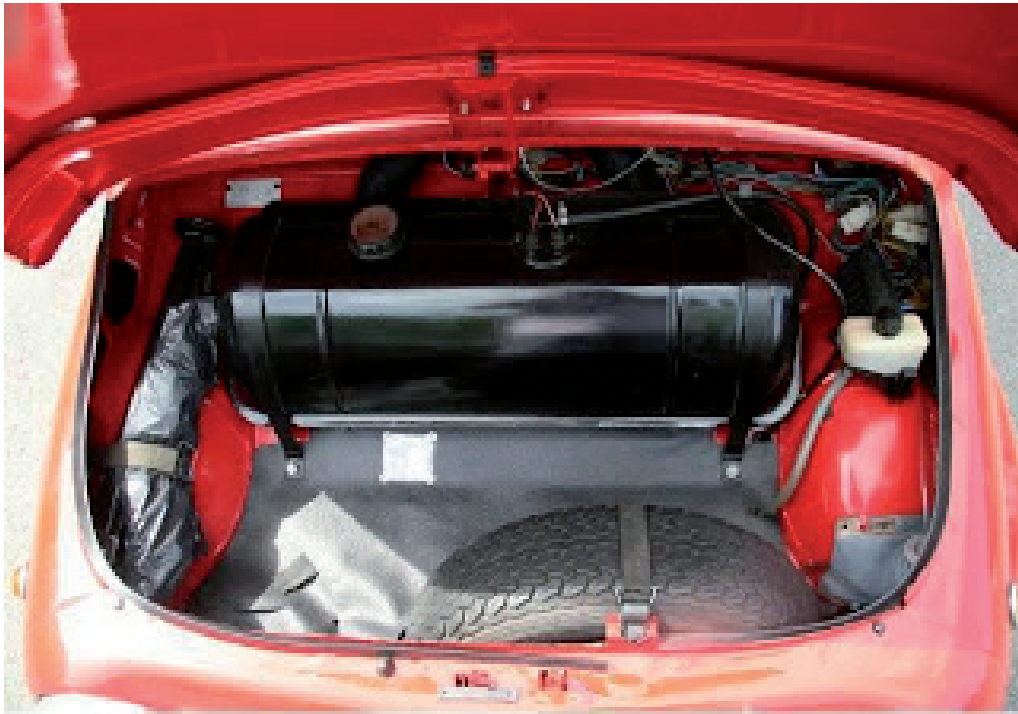
Under the bonnet. This is what you see with the bonnet opened: petrol tank behind the dashboard, spare wheel tucked into the well behind the bumper with the battery next to it (but hidden) and that minuscule space on top for a stuff bag. The new retro-Fiat 500 has the engine here. Credit: Otoreview.blogbot.com .
